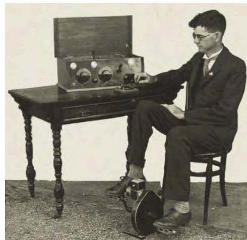
Mr. Alfred Traeger transmitting by a pedal-powered wireless, ca. 1929
